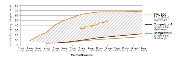
When taking the ratio of the magnets' load capacity in graph A and their dead weight into account, the hatched 'performance gain' shows the efficiency of ALFRA TML magnets in contrast to their competitors.
