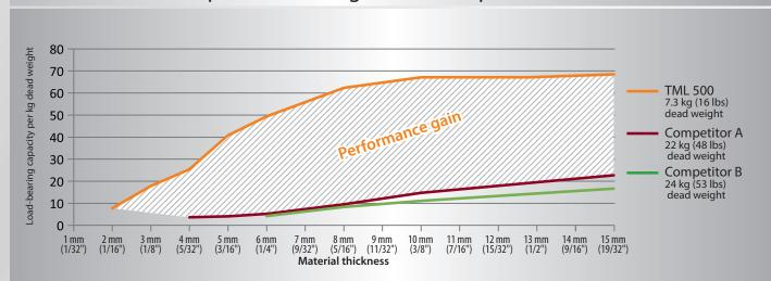
When taking the ratio of the magnets' load capacity in graph A and their dead weight into account, the hatched performance gain' shows the efficiency of TML magnets in contrast to their competitors.
