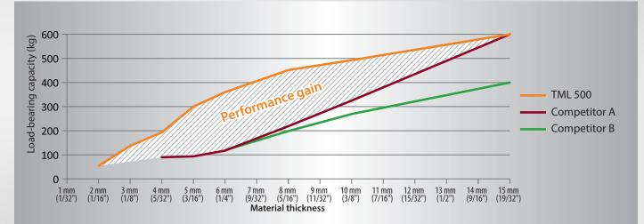
A comparison of the performance data of the TML 500 and two conventional magnets reveals how powerful the TML 500 is, especially when used on thin materials.
