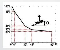
You can calculate the maximum load-bearing capacity of your magnet, including the 3:1 safety factor, on the basis of the load-figure that corresponds to the direction.
