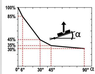
**Maximum load weight with 3:1 safety factor = 360 kg x 100 % x 30 % = 108 kg**
